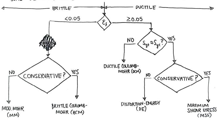
THE MAXIMUM-SHEAR-STRESS (MSS) THEORY PREDICTS THAT YIELDING BEGINS WHEN THE MAXIMUM SHEAR STRESS IN ANY ELEMENT EQUALS OR EXCEEDS THE MAXIMUM SHEAR STRESS IN A TENSION-TEST SPECIMEN OF THE SAME MATERIAL WHEN THAT SPECIMEN BEGINS TO YIELD. (ALSO KNOWN AS THE TRESCA OR GUEST THEORY)
