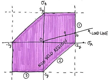
\* IF POINT A RERESENTS THE STRESS STATE OF A CRITICAL STRESS ELEMENT PLOAD LINE OF A MEMBER, AND POINT 6 REPRESENTS THE STRESS STATE OF THAT SAME ELEMENT AT THE CRITICAL LOAD, THEN THE FACTOR OF SAFETY GUARDING AGAINST YIELD AT POINT a IS
